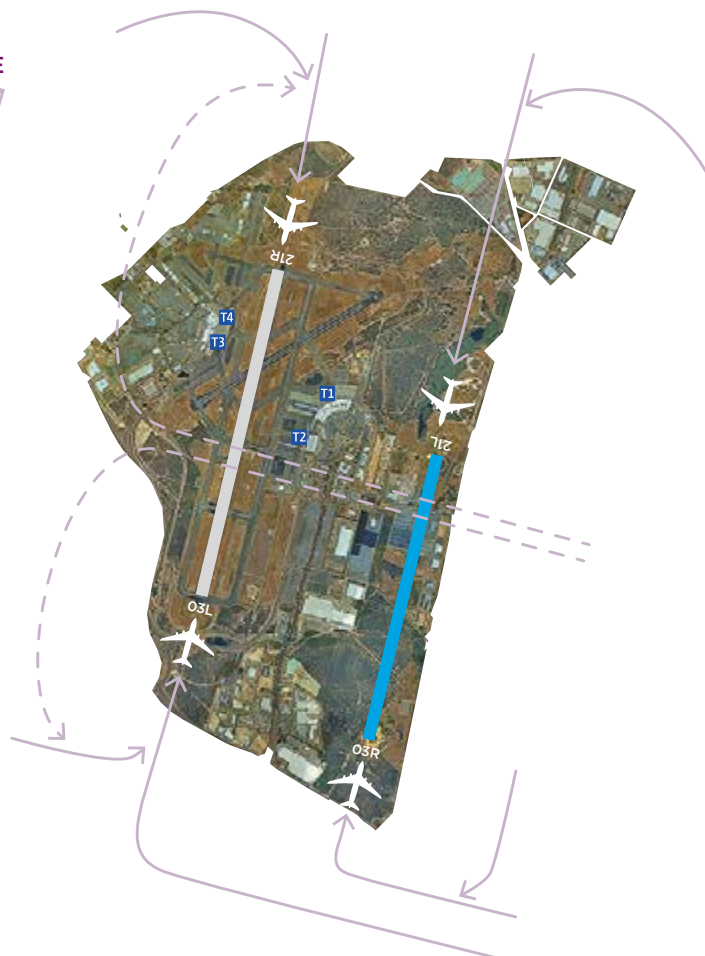
Figure 21-2 Compass departures and terminal arrivals concept of operation for parallel runway operations at Perth Airport Source: Perth Airport
