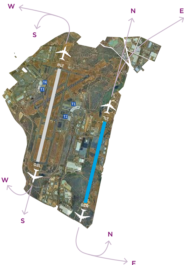
Figure 21-2 Compass departures and terminal arrivals concept of operation for parallel runway operations at Perth Airport Source: Perth Airport
