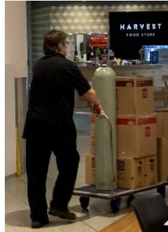
Cylinder not securely tethered during transport
